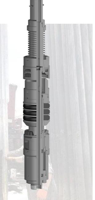
The AS Retrievable Bridge Plug is a high pressure plug for multiple zone and selective single zone operations such as acidizing, fracturing, cementing and testing. It features a large internal by-pass to reduce swabbing when running and retrieving. The by-pass closes during the setting of the plug and opens prior to releasing the upper slips to equalize pressure when unsetting. The by-pass is located directly below the upper slips to help wash debris when the by-pass is open.
