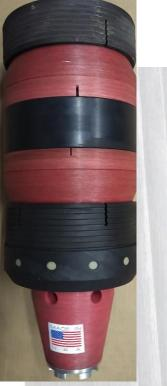
BS Composite Cement Retainers and Bridge Plugs (Patent Pending) provides a cost-effective alternative as a dependable tubing or wireline set drillable retainer. The packers are built from composite materials, aluminum, and rubber to give remarkable drill times, less drill bit wear, and less formation damage. One-piece heat-treated slips provide secure setting.
