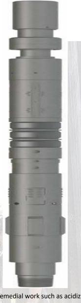
The Crest III Packer is a weight set service packer for high-pressure remedial work such as acidizing, fracturing, and squeeze cementing. It sets with minimal tubing manipulation and will withstand differential pressure from above or below.
