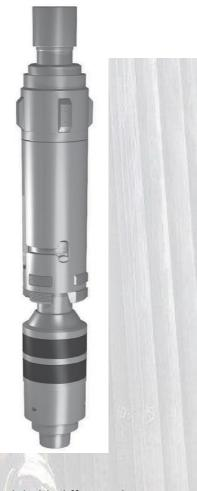
The Type T Squeeze Packer is a versatile, easy to use tension set tool which holds differential pressure from above or below. This packer is designed to run, set, reset and retrieve easily, even under adverse conditions. This packer can be set at any depth and is used when insufficient weight is available to set a compression packer. This packer is ideal for squeeze cementing, casing testing, stimulation treatments and straddle operations using a retrievable bridge plug.
